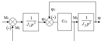
$$\begin{cases} \varphi_1 = \frac{M_1 - M_2}{J_1 p^2} \\ \varphi_2 = \frac{M_2}{J_2 p^2} \\ M_2 = C_{12}(\varphi_1 - \varphi_2) + C'_{12}(\omega_1 - \omega_2) \end{cases}$$
