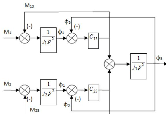
$$\begin{cases} \varphi_1 = \frac{M_1 - M_{13}}{J_1 p^2}; \\ \varphi_2 = \frac{M_2 - M_{23}}{J_2 p^2}; \\ M_{13} = C_{13}(\varphi_1 - \varphi_3); \\ M_{13} = C_{23}(\varphi_2 - \varphi_3); \\ \varphi_3 = \frac{M_{13} + M_{23}}{J_3 p^2}; \end{cases}$$
