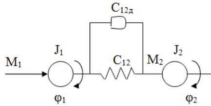
$$\begin{cases} \varphi_1 = \frac{M_1 - M_2}{J_1 p^2} \\ \varphi_2 = \frac{M_2}{J_2 p^2} \\ M_2 = C_{12}(\varphi_1 - \varphi_2) + C'_{12}(\omega_1 - \omega_2) \end{cases}$$
